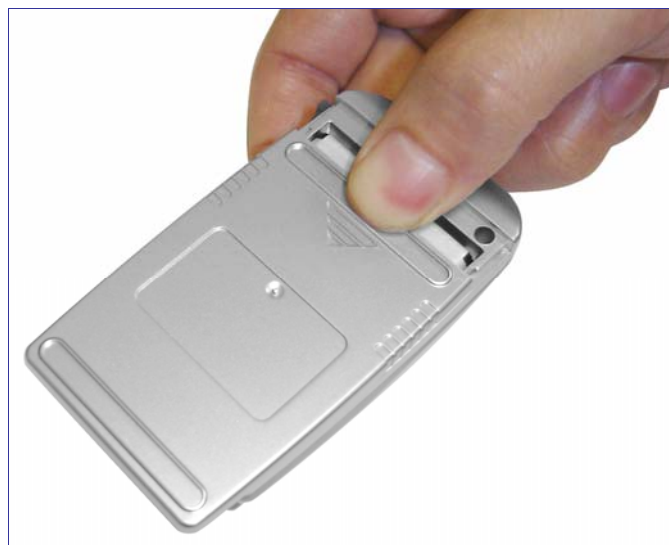
Figure 1 , Open the cover of battery
