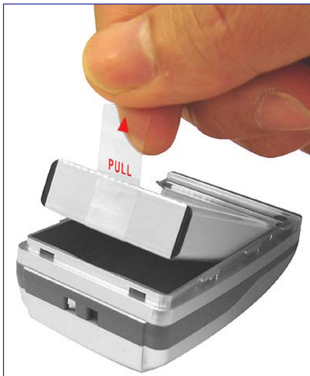
Figure 2, Take out the battery with pull tag
